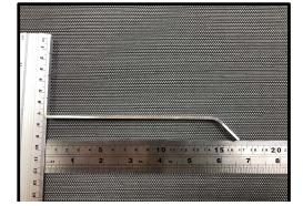
Shelf for 110mm<sup>2</sup> Headbox and 150mm<sup>2</sup> for minimal 70mm x 220mm coverage
